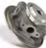
Bearing Housing Roughing and Finishing
